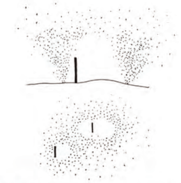
Fig. 3: Spaces are formed by the evaporation of the mist through heated screens.
