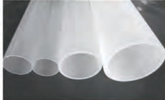
In this project, we propose to use frosted polycarbonate tubes as the 'reeds' of the project, its main building material.
