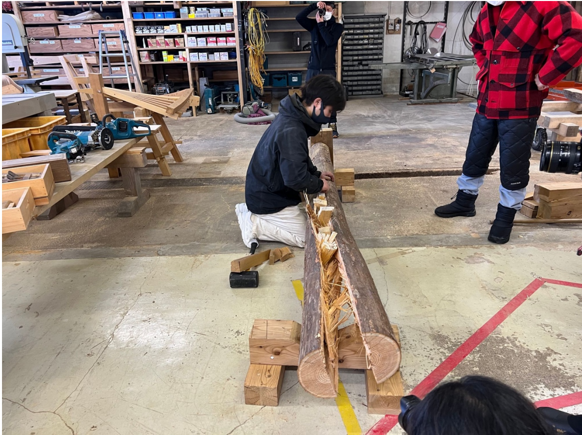
Photo 7: Larch that does not crack easily, but rather splits
