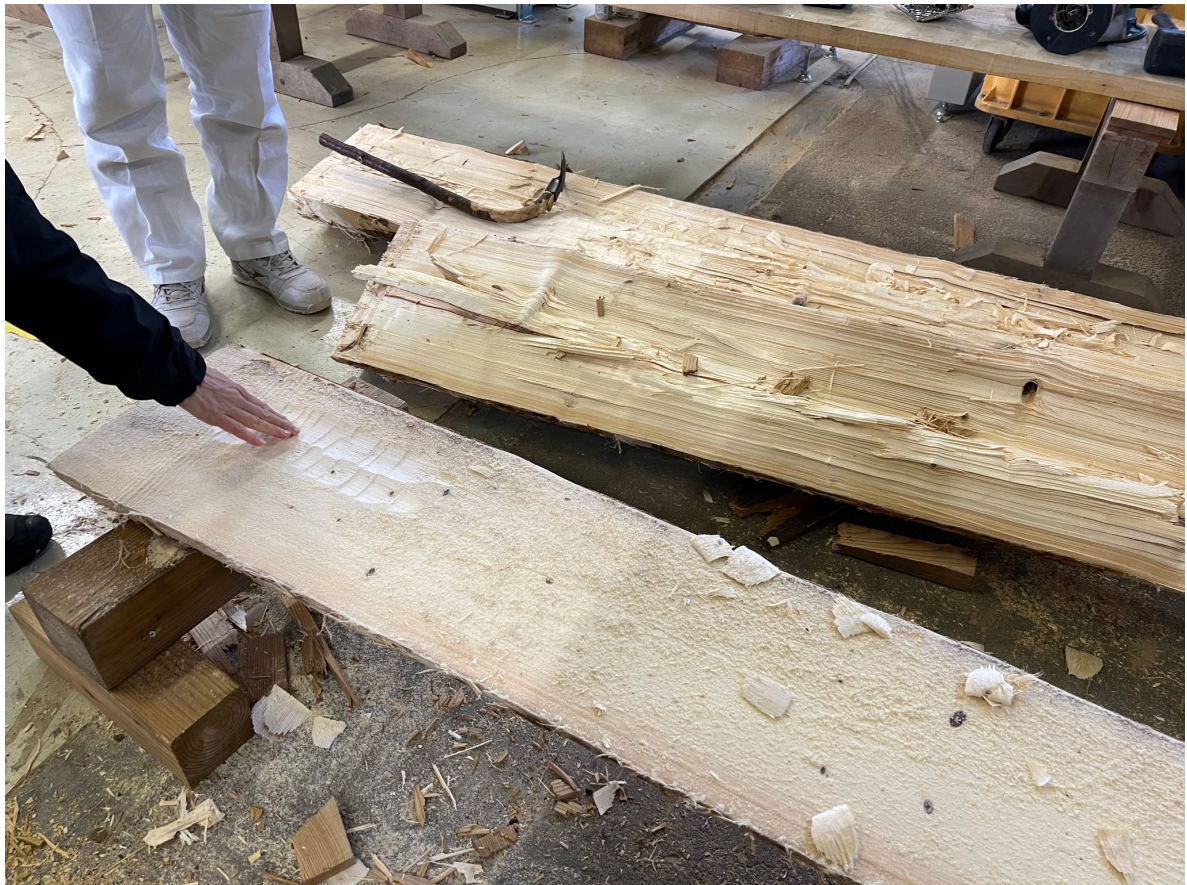
Photo: Cross-sectional comparison of split and ground Ezo spruce, and re-reading the meaning of the tools used (in this case, a hatchet).
